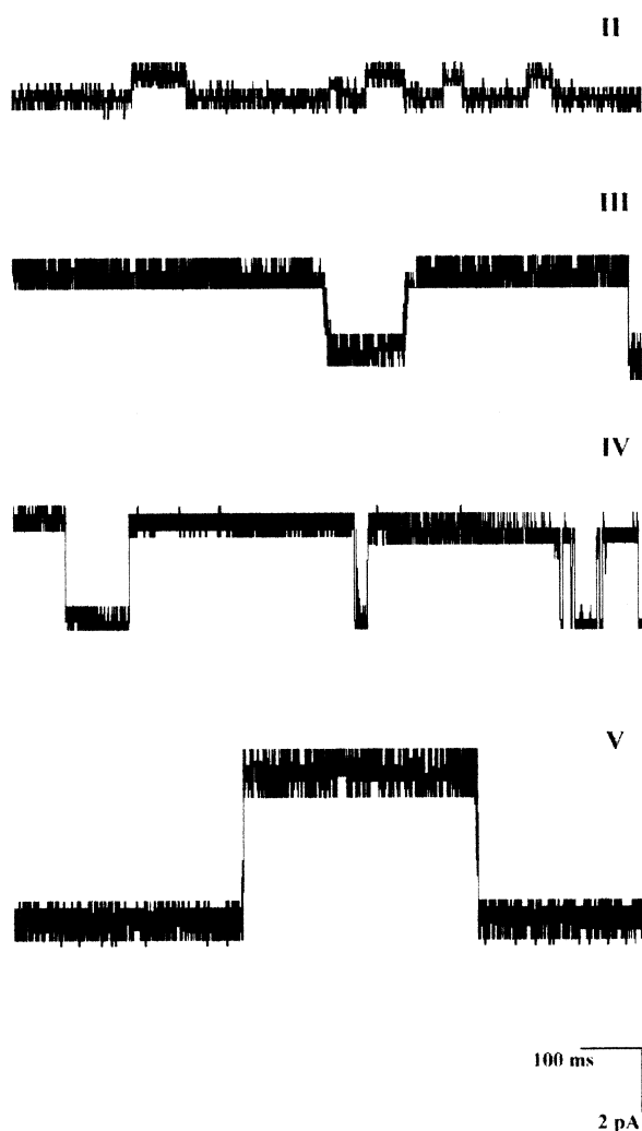
Fig. 2. A typical record showing four types (II, III, IV, V) of amphotericin B channels in the absence of sterol in a DMPC bilayer.
